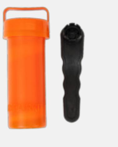
If you notice air leaking from the valve, this is easy to fix using the supplied spanner in your repair kit. Remove the valve dust cover and insert the crown shaped end of the spanner into the valve. Turn the spanner clockwise until tight to reseal.
